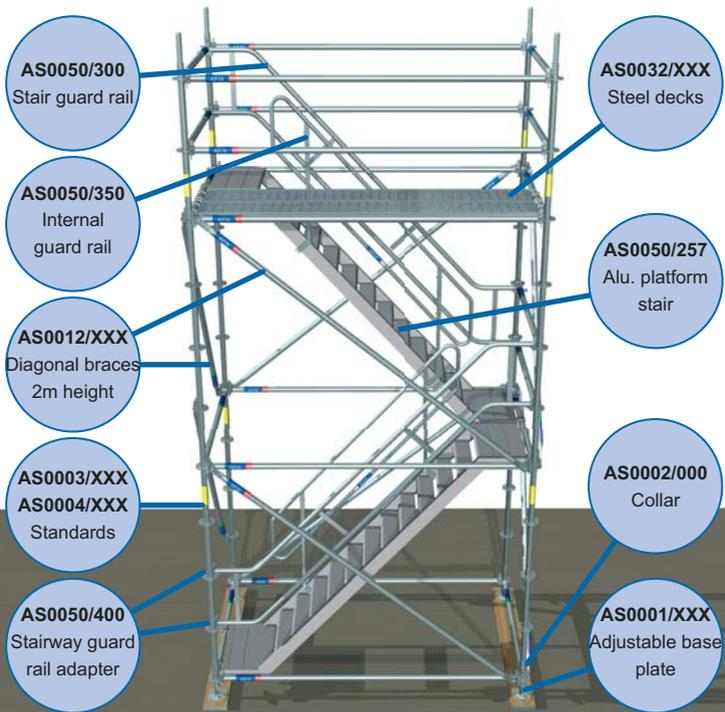
FAST FIX access ladders assembly guide
